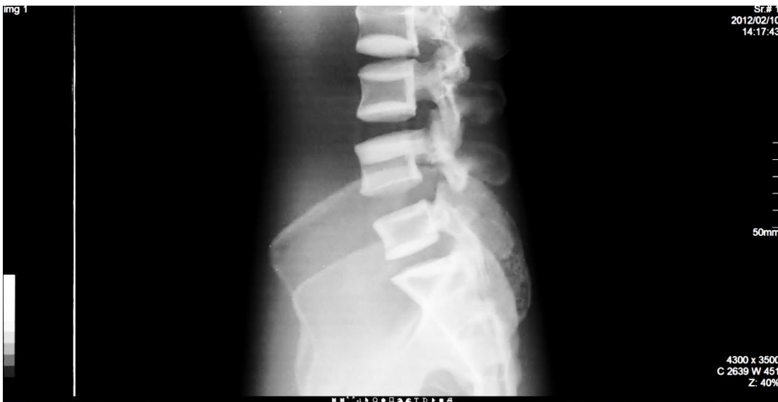
Figure 7. Example of horizontal lines from a faulty Y-axis motor or an incorrect stage alignment.
