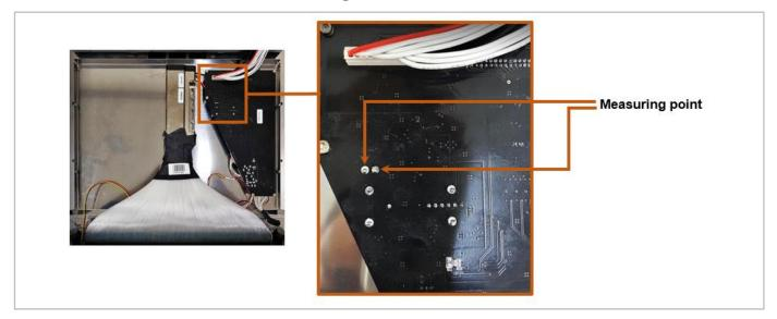
Measure the voltage DC on the photo module board during scanning only for FireCR Spark.
